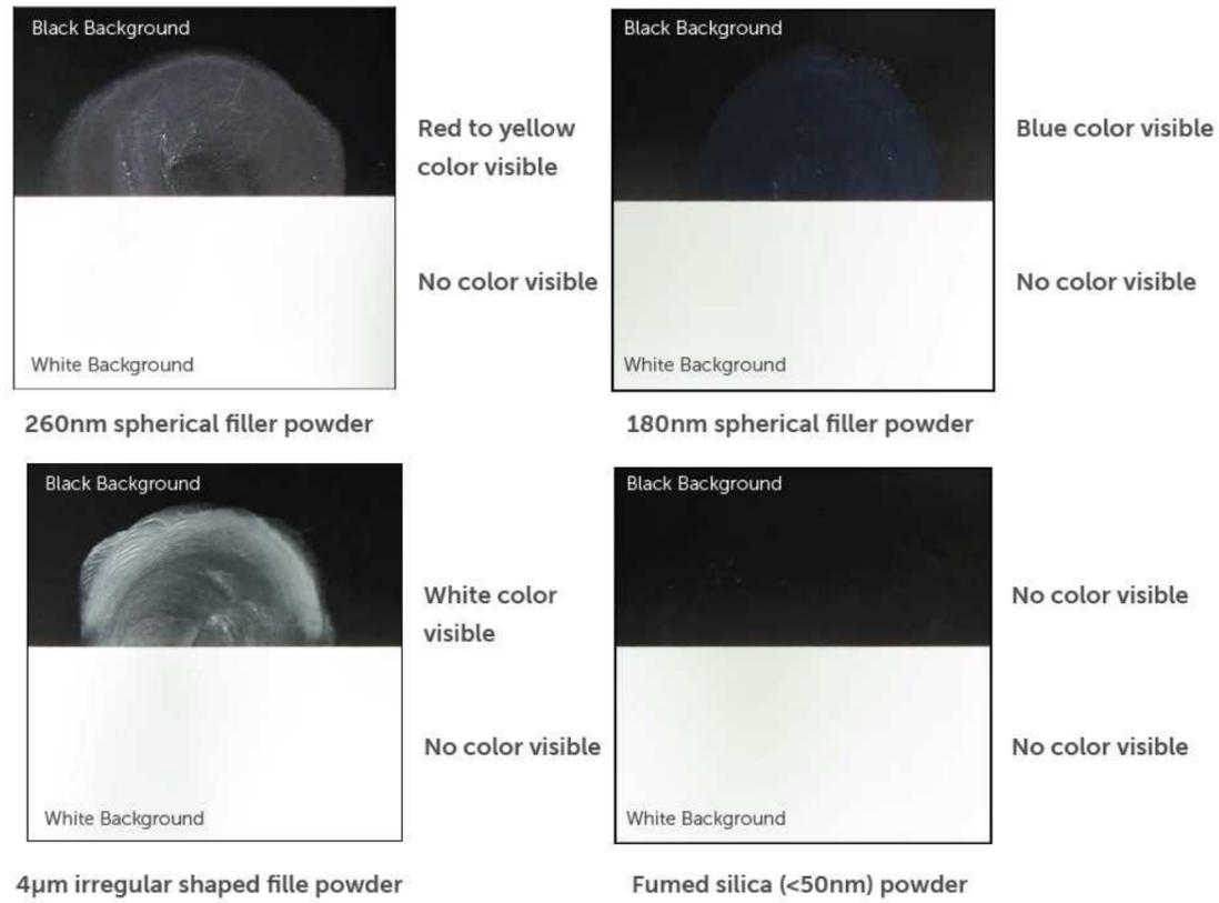
Fig. 7 Relationship between particle size and structural color phenomenon
