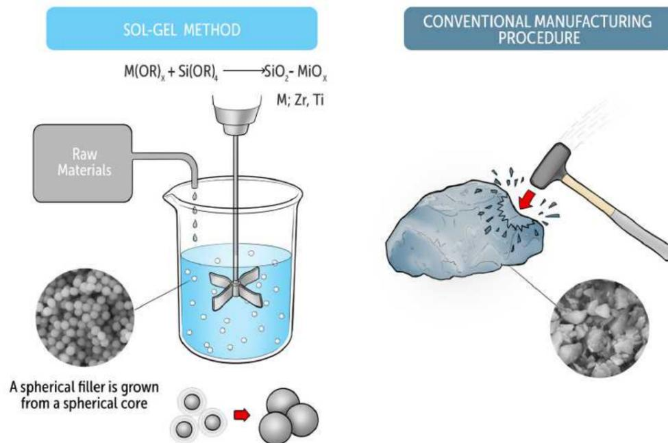
Fig. 8 Sol-Gel Method vs conventional filler method
