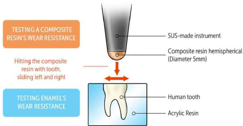
**Fig. 22 Method of testing wear resistance**
