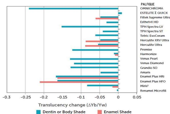
Fig. 29 Change of translucency before and after polymerization
