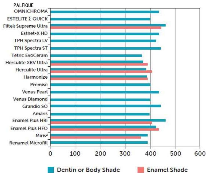
Fig. 21 Compressive strength (MPa)
