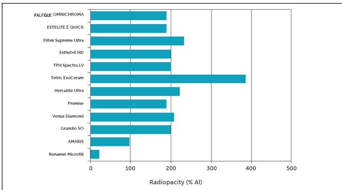
Fig. 30 Radiopacity of composite resins
