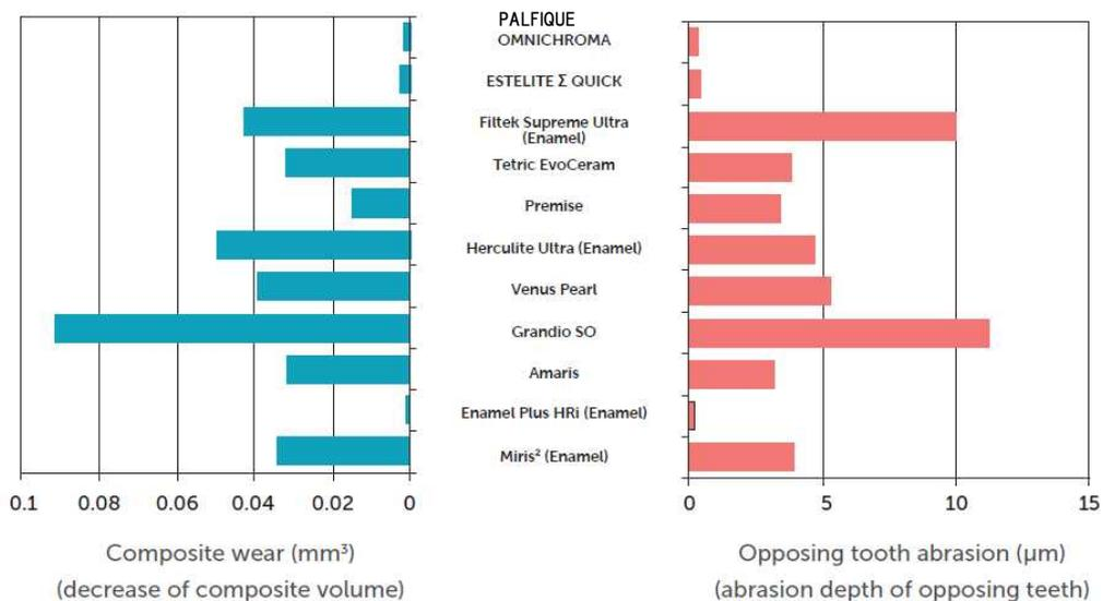
**Fig. 23 Wear resistance (50,000 cycles)**
