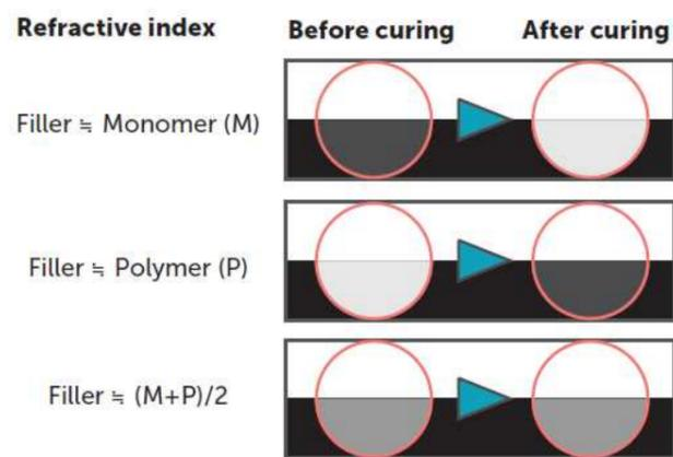
Fig. 11 Relationship with refractive index and translucency
