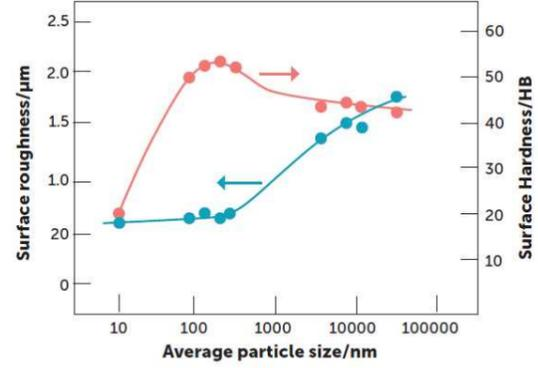
Fig. 10 Correlation between particle size, surface roughness, and surface hardness
