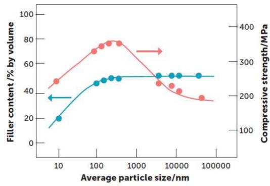
Fig. 9 Correlation between particle size, filler content, and compressive strength
