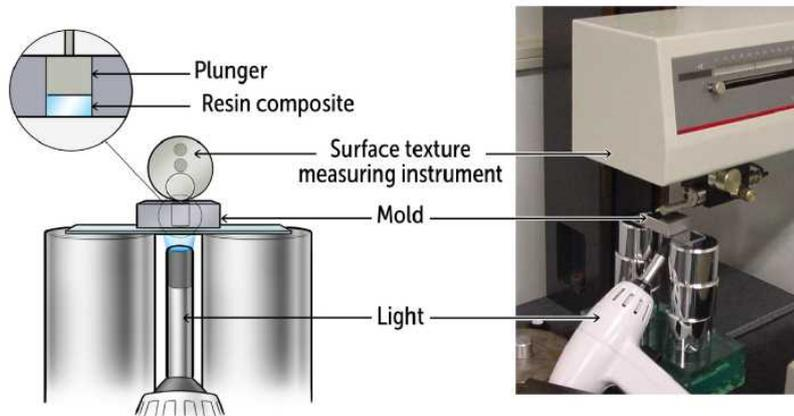
**Fig. 24 Method of measuring polymerization shrinkage**
