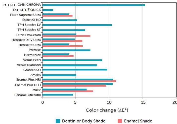
Fig. 28 Change of color before and after polymerization
